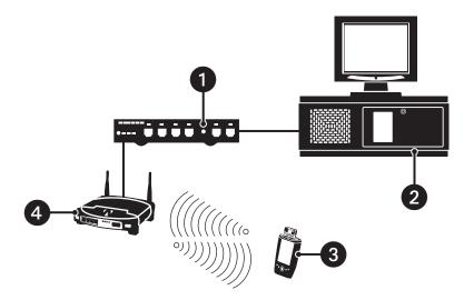
Figure 185. PDA-to-DVR Wireless Networking Example
